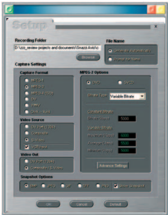
▲ The setup screen gives options for the format to encode to, input source, output signal and still image capture format
